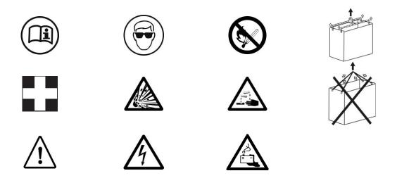
Labelling may vary due to application and dimension of the Battery. The manufacturer, respectively the importer of the batteries shall be responsible for placing the symbols (a minimum size is specified). In addition, consumer/user information on the significance of the symbols may be attached.
